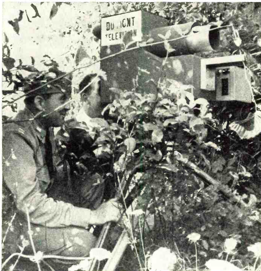
The Iconoscope camera used in the Army maneuvers. All power came from batteries and portable generators.
